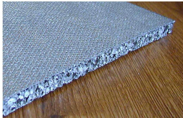
Figure 3: Foamed panel (up) reinforced in the surface with stainless steel mesh (down)
