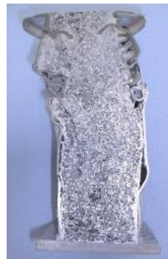
Fig. 4. The foam density giving maximum energy absorption depends on allowed stress level (left). The foamed motor carrier after frontal impact (right)
