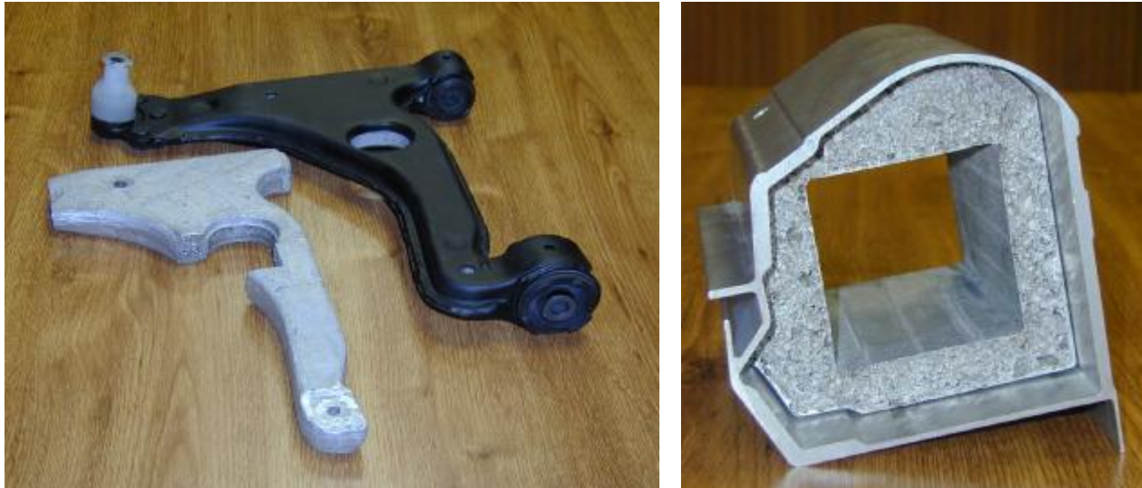
Fig. 5. Suspension and car body part reinforced with aluminium foam inserts
