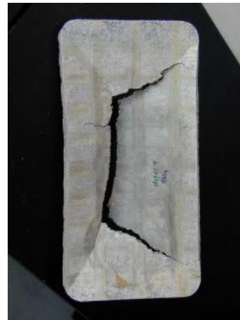
Figure 12: Bending of foamed panels under surface loading (right- broken plain foam panel).
