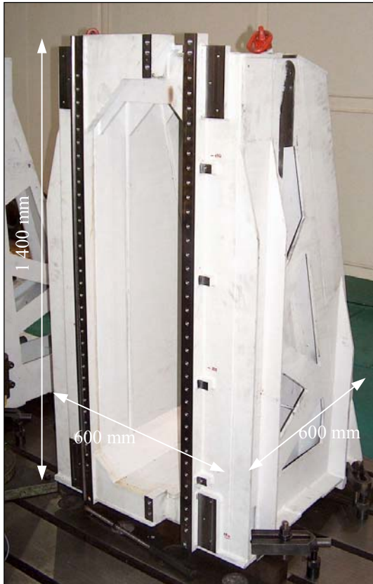
Fig. 4. Realised welding construction.
