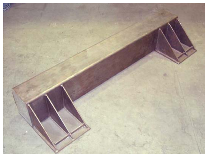
Fig. 2. : Cross beam ( foamed out) of the laser cutting unit
