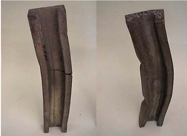
Fig.3. Beams made of aluminium foam after buckling (left fractured plain foam, right buckled reinforced foam of similar weight)
