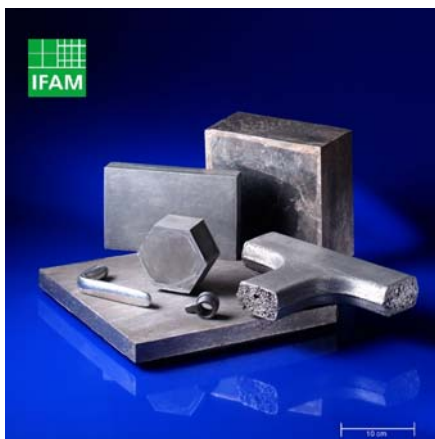
Fig. 3. Aluminium foam parts produced in a foaming mould by the powder-metallurgical IFAM process
