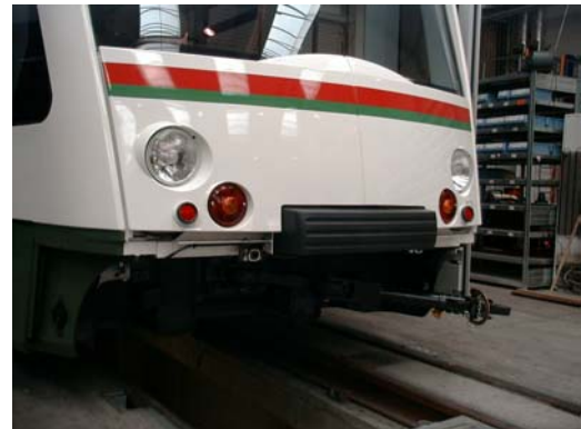
Fig. 11. Frontal view of suburban railcar with frontal crash energy absorber consistent of aluminium foam and polymer foam both covered by a rubber surface layer
