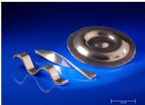
Fig. 5. Aluminium foam sandwich (AFS) formed and twisted before foam core layer expansion
