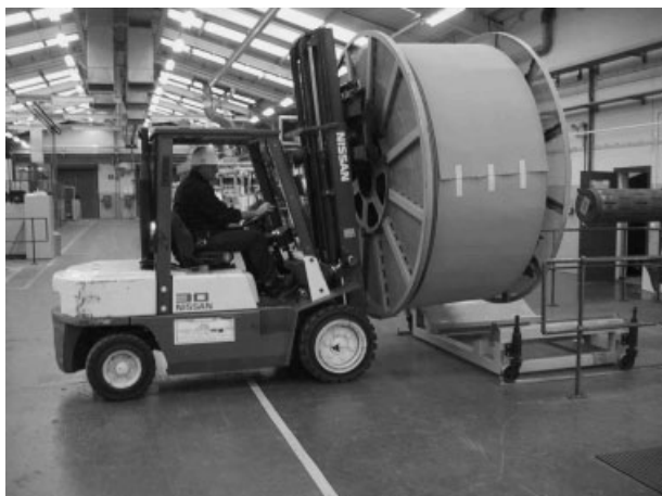
Fig. 1. As-produced Ni foam coil shown in transit between plating and sintering operations.
